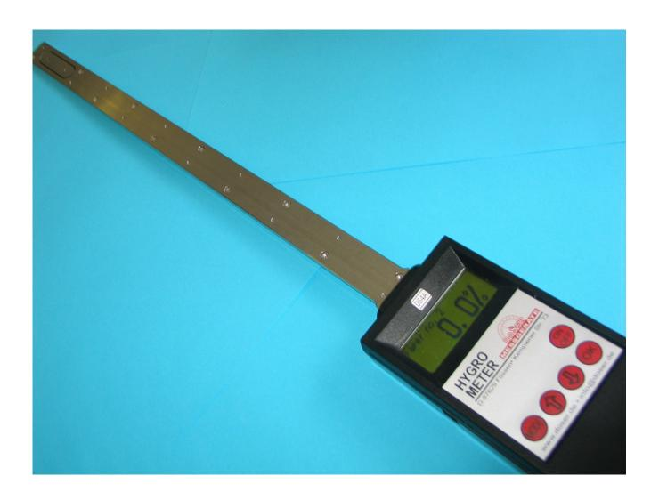
The DS3U can be used for measuring moisture in stacks of veneer, corrugated boards, single card board sheets, ...
